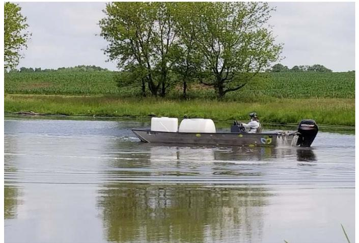
(Left photo) Tanks of liquid aluminum sulfate along wetland shoreline. These tanks are then loaded into a boat, and the alum is pumped into the water through injectors off the back of the boat (right photo). The Moody Lake round barn park will be used as a staging area and boat launch site for the whole lake alum treatment this fall.
