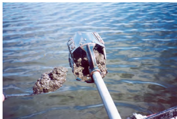
Figure 2. Soil auger used to collect lake sediments in water depths to 10 feet.
