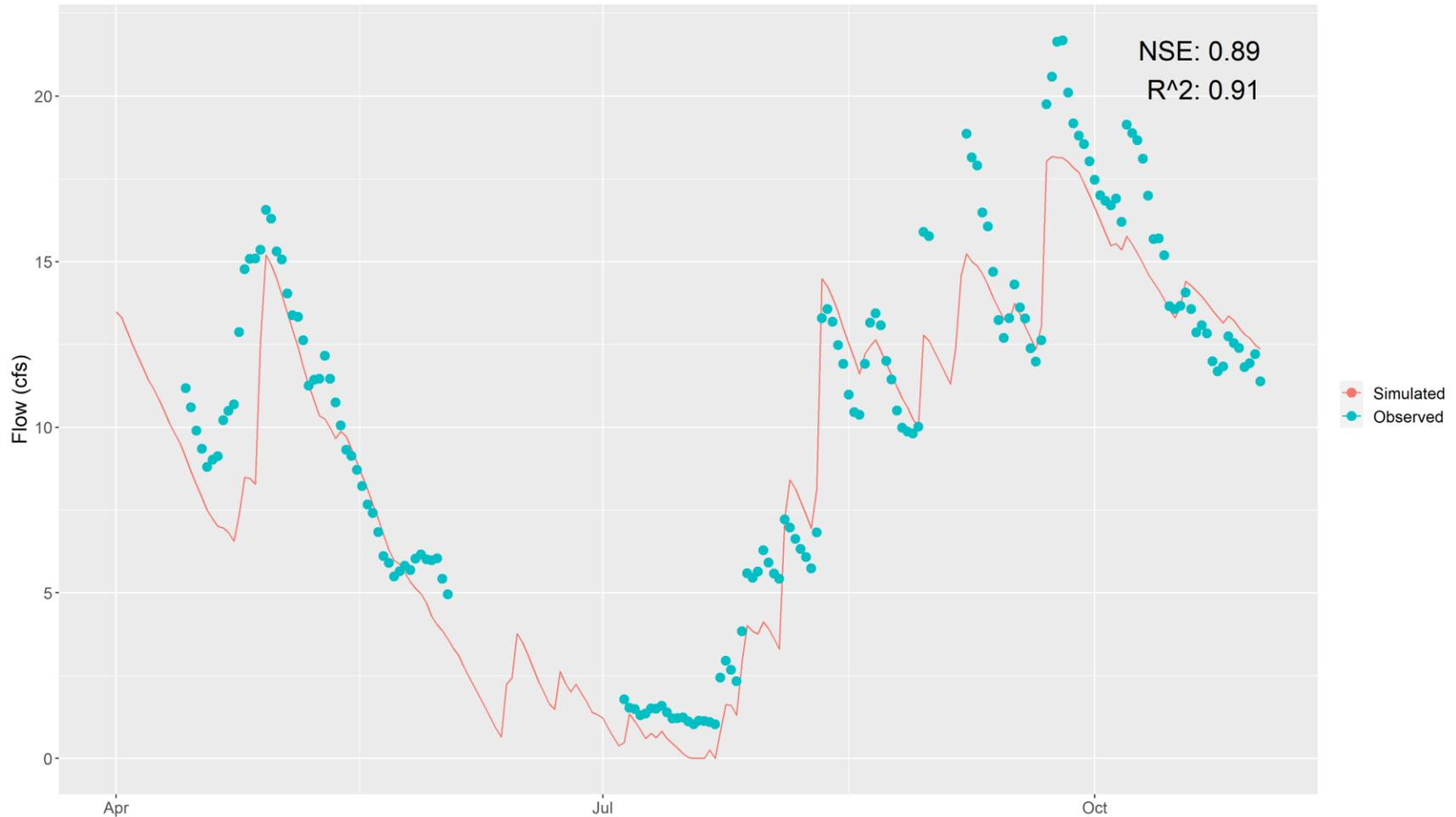
The FL1 monitoring station is located just downstream of the culvert crossing at North Shore Drive, where outflow from Forest Lake becomes the headwaters of the Sunrise River. No additional changes to the model were necessary to match the observed data. Total volume for the model was 91% of the observed volume (excludes month of June when monitoring station was offline).
