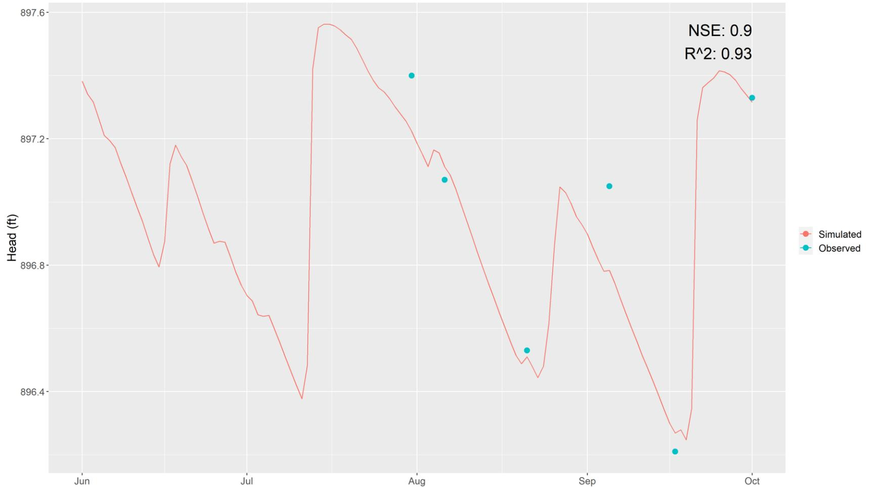
To match observed levels on Birch Lake, the modeled channel from the lake downstream to the July Avenue crossing culvert was widened by 8 feet to provide additional capacity. The original capacity was estimated based on two surveyed cross-sections located roughly 100 feet upstream of the culvert and may not have been reflective of the overall channel cross-section.
