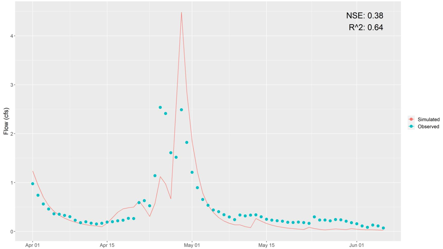
The 208<sup>th</sup> Street Pond monitoring station is located at the end of the ditch from Ditch West, at the intersection of 208<sup>th</sup> Street and 209<sup>th</sup> Street North. The outlet from this stormwater pond drains directly to Shields Lake. No additional changes to the model were necessary to match the observed data. Total volume for the model was 92% of the observed volume.
