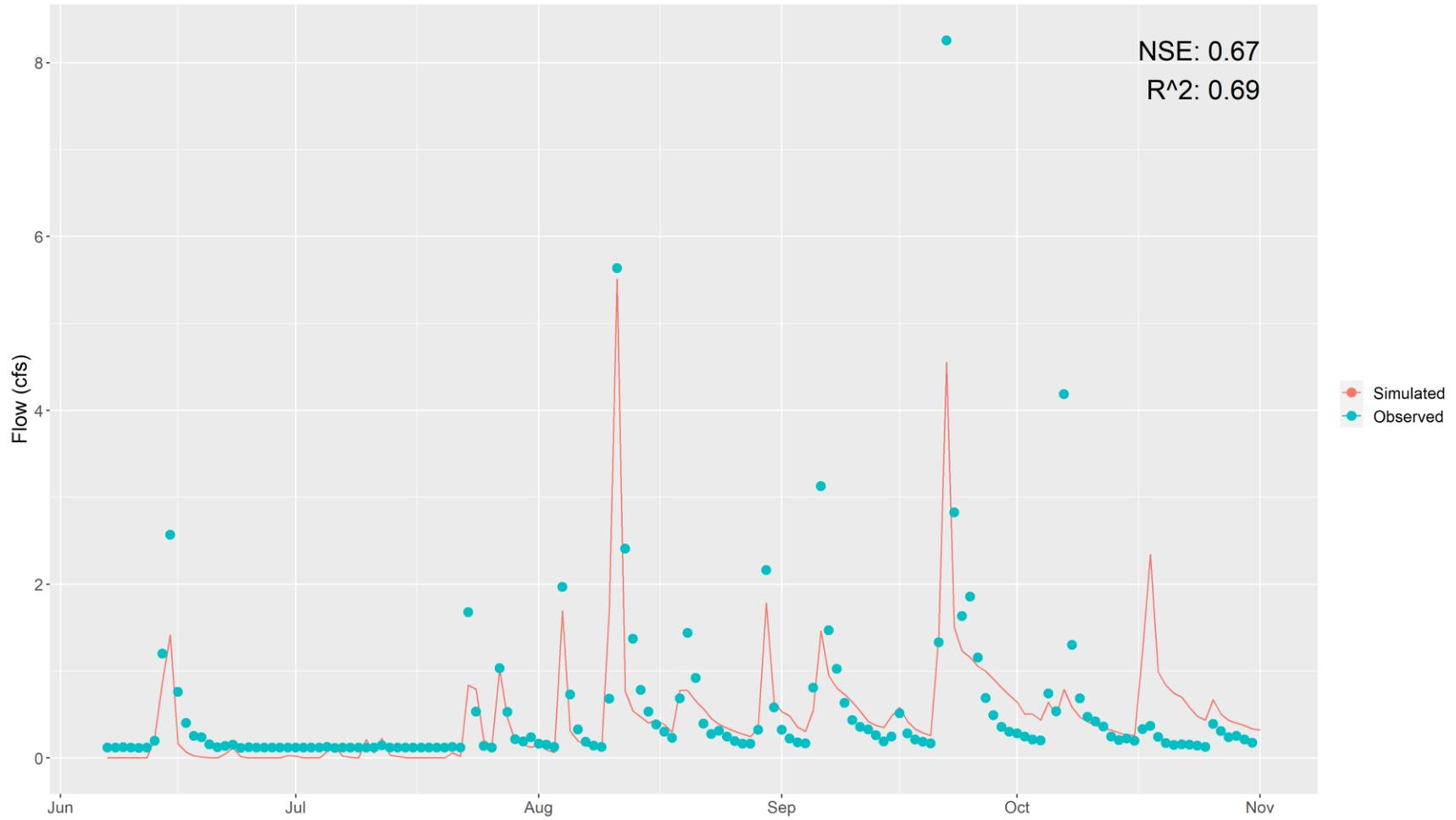
The FL8-D monitoring station is located at the downstream end of a large stream tributary, where a pipe draining the Castlewood golf course outlets into Forest Lake just east of 12<sup>th</sup> Ave SE. No additional changes to the model were necessary to match the observed data. The graphic shows small flows with a good NSE and R<sup>2</sup>. Total volume for the model was 87% of the observed volume, which is considered a good match.
