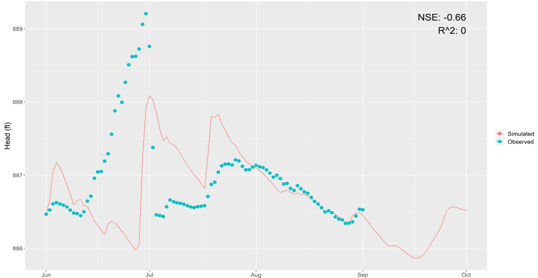
A beaver dam was observed on June 12 and was cleared on July 1, resulting in the large increase in elevation in mid-June and then sudden drop when the dam was removed (see graphic above). Removal of the beaver dam impacted the sensor's response to a large rainfall event occurring June 28-30. The monitored data in the graphic shows a sudden drop in elevation instead of a more logical and expected days-long drop in water elevation as water levels peak and then slowly recede from the storm.
