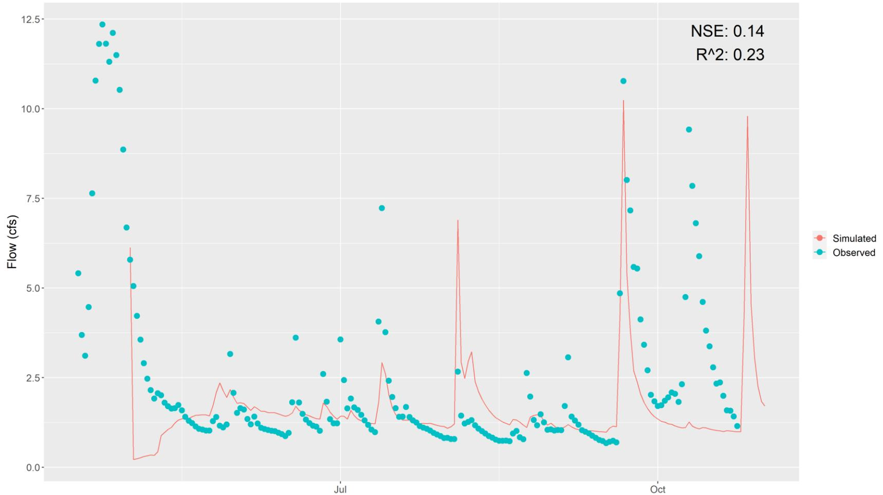
The FL10 monitoring station is located at the downstream end of the JD6 ditch system where the ditch crosses Scandia Trail N. No data was available for this monitoring station in 2016, so 2018 was used as a validation year with no adjustments made to the tributary catchments. Total runoff volume for the model was 92% of the observed volume.
