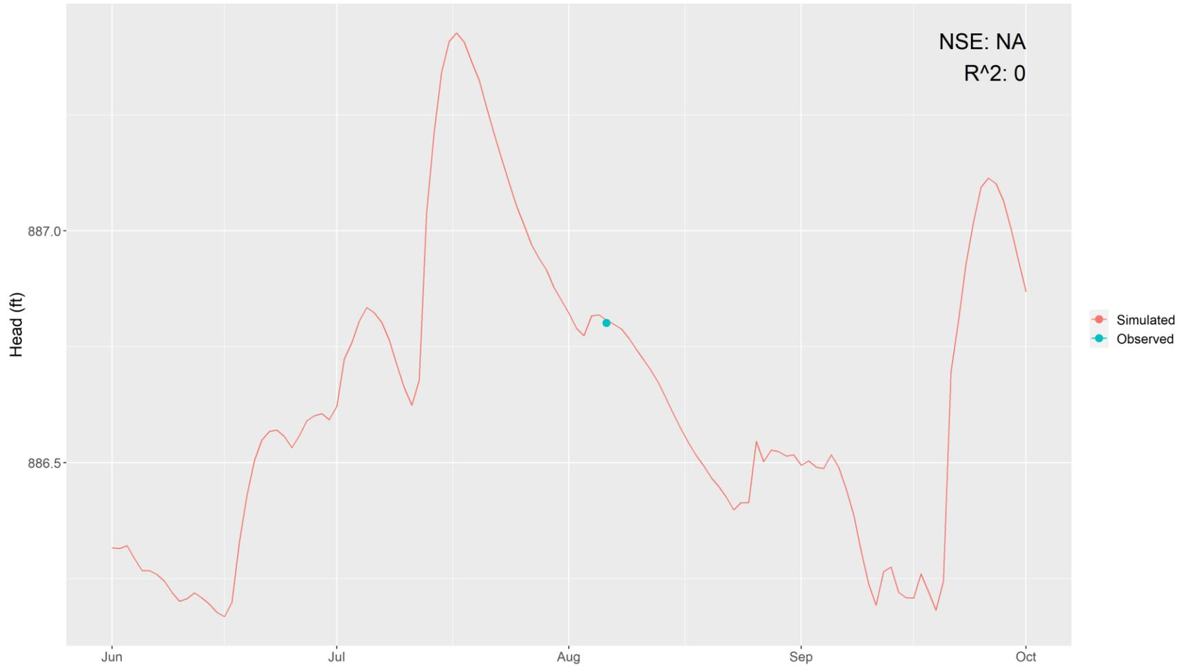
No data was available on Little Comfort Lake in 2018 to use for setting downstream boundary conditions. Instead, monitoring data from the Comfort Lake outlet @ Wyoming Trail station was adjusted to match observed levels on Comfort Lake as shown in the image above. Comfort Lake had two other data points in 2018, but both were before June 1 and excluded from the simulation period.
