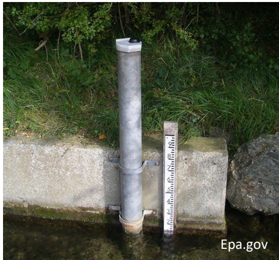
Figures 4 and 5. Stilling wells, staff gages (left panel), and level loggers (right panel) are essential tools in sequential diagnostic monitoring.
