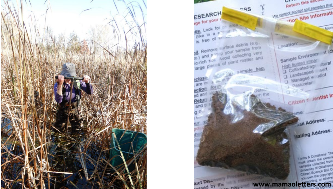
Figure 12. Soil borings being collected using a hand auger in the Bone Lake dairy wetland (left panel) and a representation of the soil samples collected (right panel).
