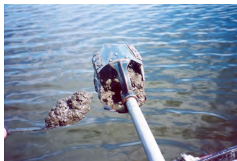
Figure 1. Soil auger used to collect lake sediments.
