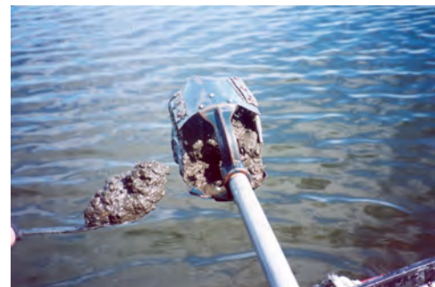
Figure 1. Soil auger used to collect lake sediments.
